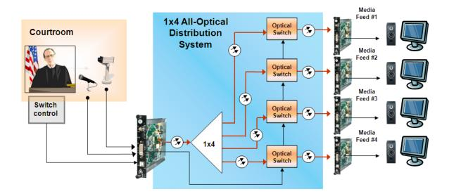
All-optical routing and switching adds capabilities to the transport and routing system not presently available in copper-based systems. By keeping the signals in the optical domain, the quality of the signals (video & audio) is maintained since conversion to and from the electrical domain is done primarily at the end points of the system.
